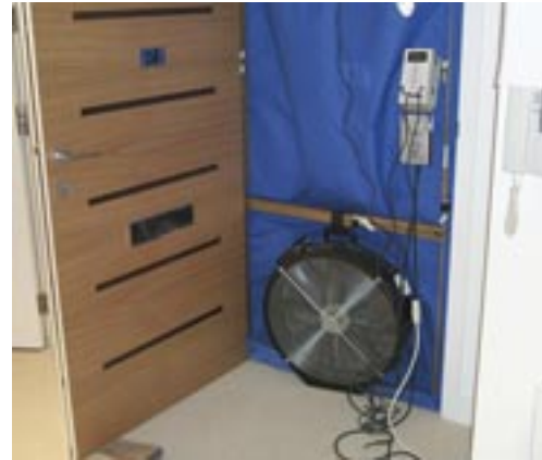
Figure 21 Air tightness testing equipment.
